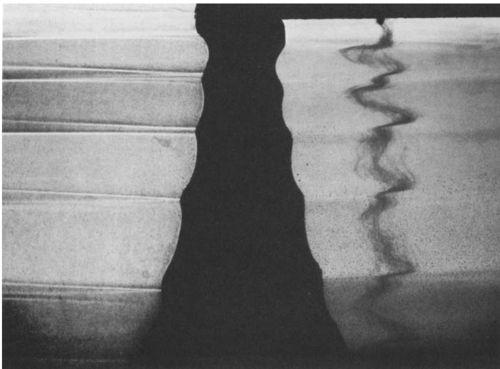
FIGURE 10. A crystal column produced by cooling an initially homogeneous solution of \text{Na}_2\text{CO}_3 at a central pipe. Upflow in the boundary layer due to crystallization has produced stratification and layering and associated 'scallop' on the crystal surface. The left of the picture is a shadow-graph and the right shows a dye streak against diffuse back lighting, with the distortions indicating the motion in the layers.
